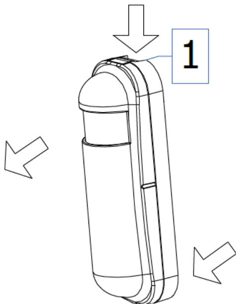
Replace the new battery and install the cover back.
